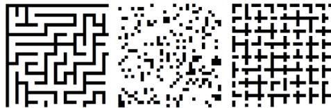
Figure 12: Types of maps used in the experimental evaluation. From left to right: *maze*, *random*, and *room*.
