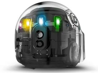
**Fig. 4.** Ozobot Evo from Evolve used for the experiments. Picture is taken from [9].
